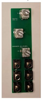
3/ Place the front panel, ensure everything is in place and solder the jacks and potentiometers.
